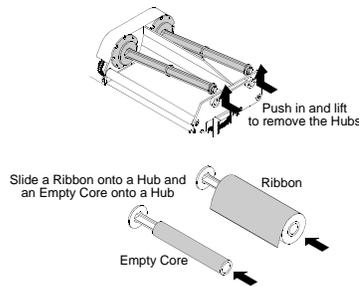
c) Replace the Hubs so that the ribbon flows as shown below:
