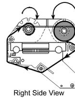
**Note:** Ensure the inked side of the ribbon faces the media and NOT the printhead.
