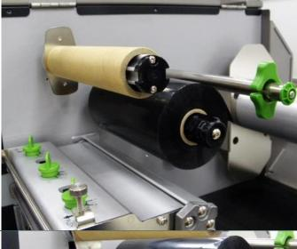
2. Install the ribbon and paper core onto the ribbon supply spindle and ribbon rewind spindle.
