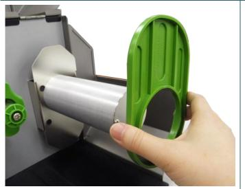
Remove the label roll guard from the label spindle.
