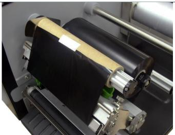
5. Stick the ribbon onto the paper core. Keep the ribbon flat and without wrinkle.
