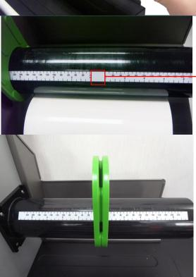
B. Make sure the width of the label. (You can refer to the ruler on the spindles.)
