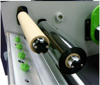
Install the ribbon and paper core onto the ribbon supply spindle and ribbon rewind spindle. Make sure the ribbon & paper core are set at the center of the spindle. (You can refer to the ruler on the spindles.)
