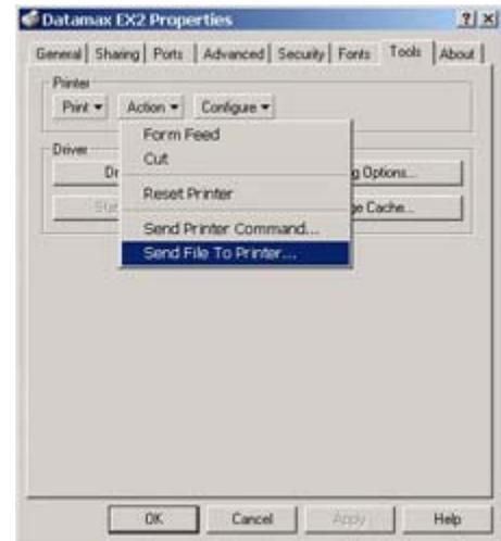
Print a Database Configuration Label via the Windows printer driver to verify your new firmware version.
