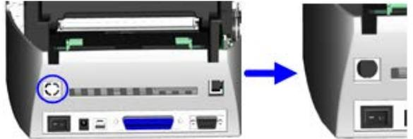
10. Put the antenna connector through the antenna bracket and then through the opening for the antenna jack as shown.
