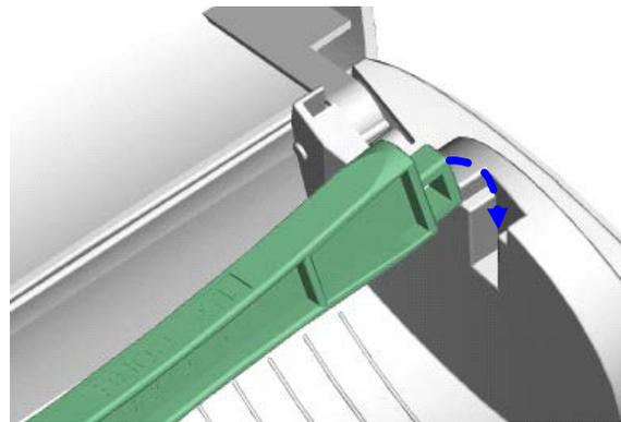
(C) Installing the label supply hub for 3" cores
