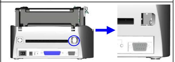
5. Secure the Ethernet module on the bracket.
