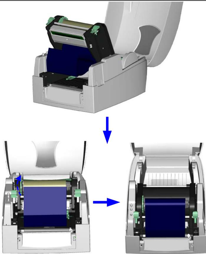
7. Close the print mechanism. Ensure the release catches click into place.
