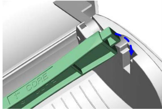
(B) Installing the label supply hub for 1.5" cores
