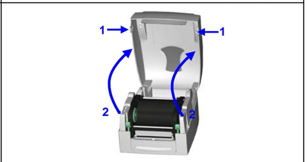
3. To remove the top part of the printer housing, gently pull the open printer cover upwards.
