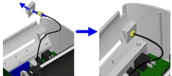
11. Put first the fixing plate and then the washer on the antenna connector. Now secure them with the nut.
