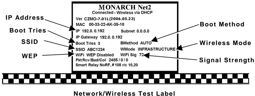
The third test label displays the settings for the IP address, subnet address, IP gateway, boot tries, boot method, SSID, wireless mode, WiFi WEP, WiFi signal, packets received, bad packets received, and packet collisions. It also lists Smart Relay information. See Chapter 2 or 3 if you need to change any of the IP or wireless settings.
