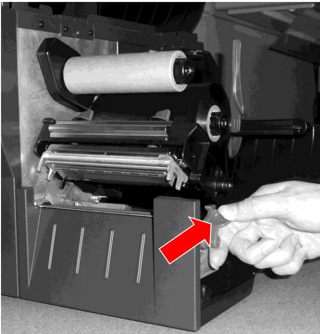
4. Push the deck lock lever back to open the pivoting deck.
