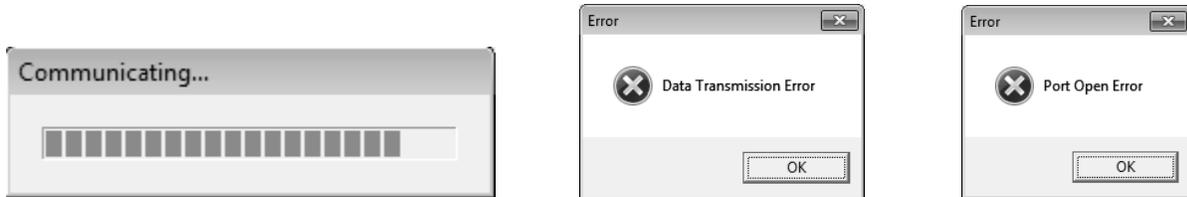
If communication problems persist, change the Tool Interface to USB. This is the easiest method of establishing communication with the printer. Once communication is established, click “Read” to upload the configuration. Check the Interface Tab settings if necessary.
