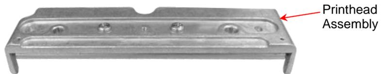
8. Connect the printhead cable and carefully lift the assembly into the pivoting deck.
