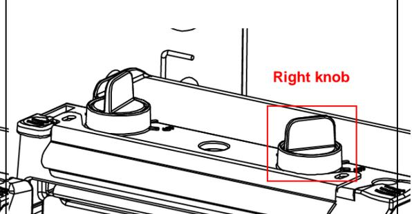
The printhead pressure adjustment knob has five setting levels. Clockwise adjustment increases the printhead pressure. Counter clockwise adjustment decreases the printhead pressure.
