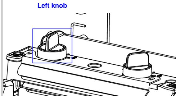
The printhead pressure adjustment knob has five setting levels. Clockwise adjustment increases the printhead pressure. Counter clockwise adjustment decreases the printhead pressure.
