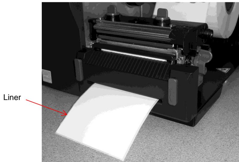
7. Use the Configuration Utility to set the printer to Peel-Off mode. Peeling will automatically start. Press the **FEED** key to test.
