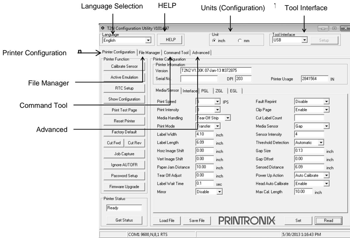
**Figure 6. Configuration Utility Components**
