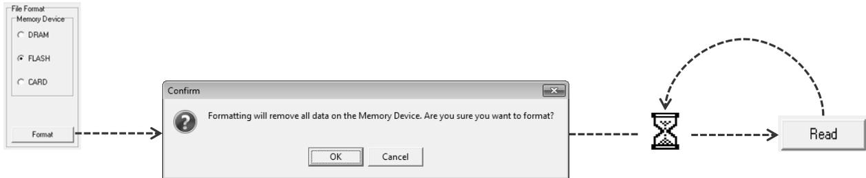
This action deletes all files in that device. Confirm whether to perform this action (see above). As shown, once the formatting process starts, the user is required to wait for the formatting to complete before continuing to use the printer. For DRAM and FLASH, this is a quick process. For SD Card, this may take several minutes. The user can click the “Read” button from the Printer Configuration tab to verify process completion. If the “Read” operation is successful, the process is complete.
