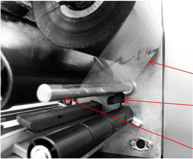
5. Thread the ribbon under ribbon guide bar and through ribbon sensor slot. (See page 25 for ribbon loading diagram or refer to diagram on printer media cover.)
