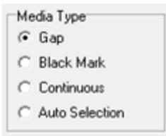
First select the Media type: Gap, Black Mark, Continuous, or Auto Selection. If the label is a continuous form, the calibration function checks for the transparency of the paper. Auto Selection can be used when the user has unique media that is not easily categorized as one of the previous selections. Auto Selection may result in a longer calibration process.
