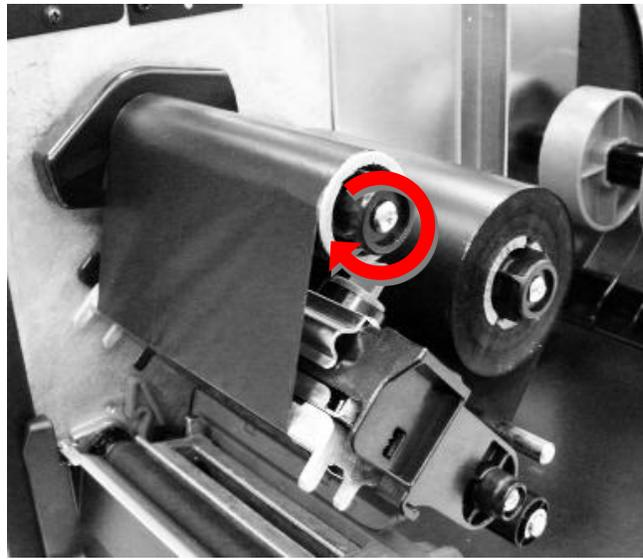
7. Rotate ribbon take-up spindle clockwise 3 to 5 full turns until ribbon is wrinkle-free.
