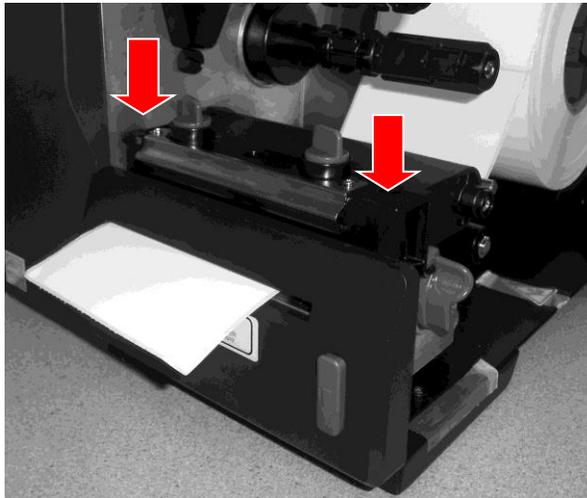
4. Close pivoting deck ensuring the latches engage properly.
