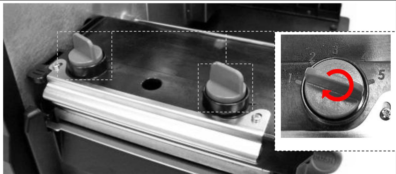
Adjust printhead pressure under these conditions:
