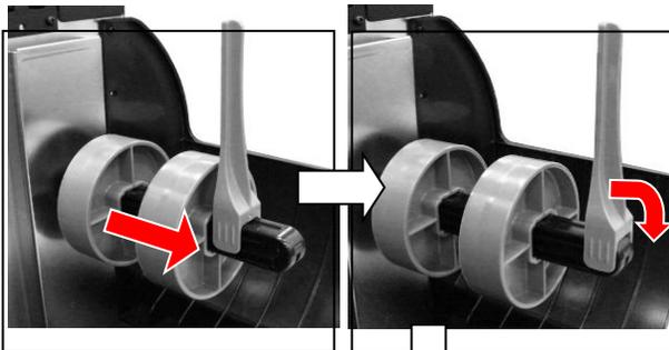
3. Move the label roll guide to the end of the media hanger then place it in horizontal position. (If paper core is 3 inches, install 3 inch core adapters on the beam.)
