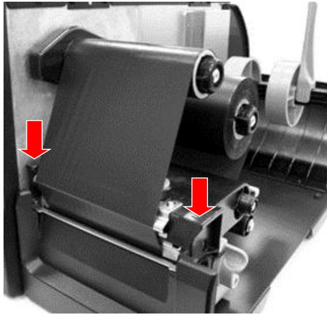
8. Push both sides of the pivoting deck down to close it, ensuring the latches engage properly.
