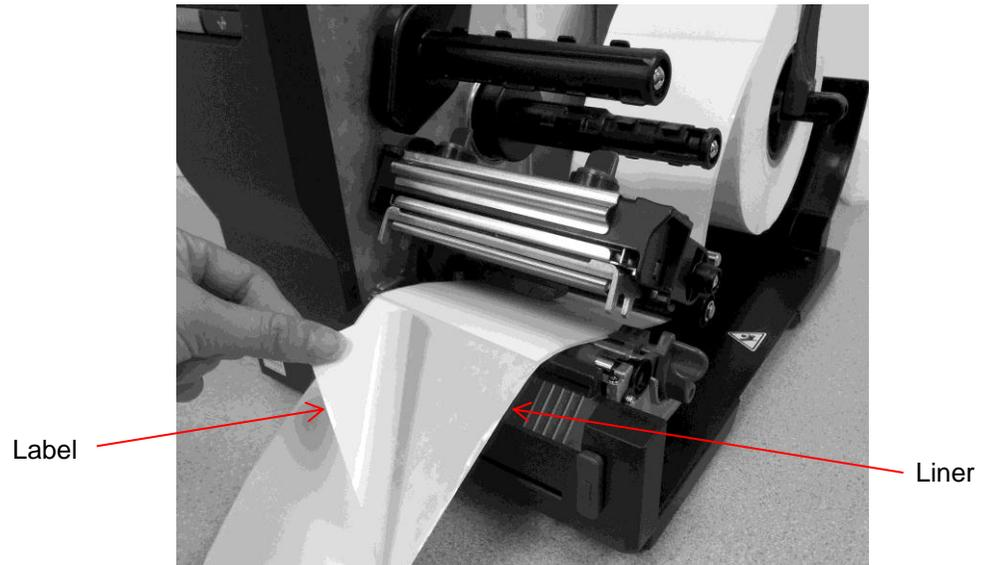
5. Feed the liner into the peel-off cover slot.
