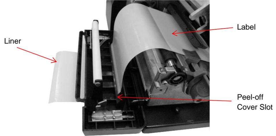
6. Close the peel-off cover and pivoting deck.
