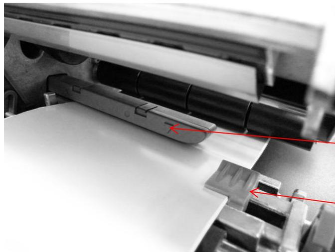
6. Adjust media width guide to fit label width. Adjust media sensor ensuring the gap/black mark passes underneath the media sensor indicator (marked by a triangle) for sensing.
