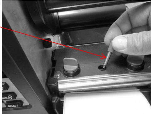
11. Open and close the pivoting deck ensuring the latches continue to engage properly.
