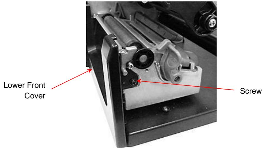
4. Remove screw on the platen right side bushing.
