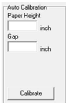
Upon clicking the “Calibrate” button, the printer will calibrate (feed) up to the value specified in “Max Cal. Length” (in Media/Sensor tab) or 10” by default.
