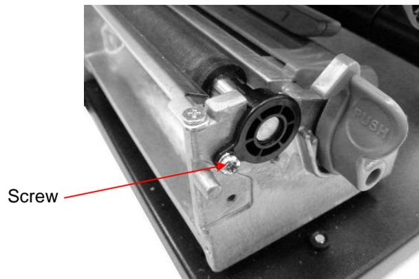
5. Disengage the platen left side bushing tab from the printer.
