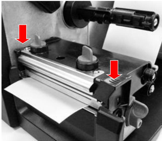
7. Push both sides of the pivoting deck down to close it, ensuring the latches engage properly.
