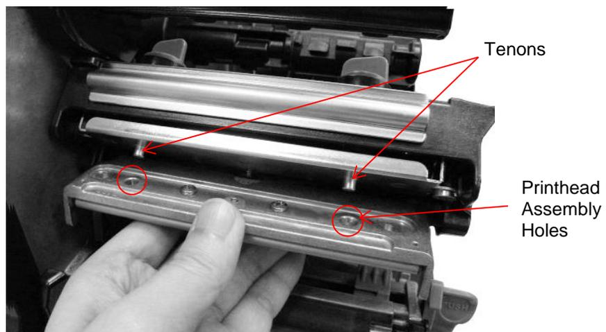
10. Close the pivoting deck and ensure the levers engage properly. Install the new thumbscrew (provided in every printhead assembly kit) to secure the printhead.
