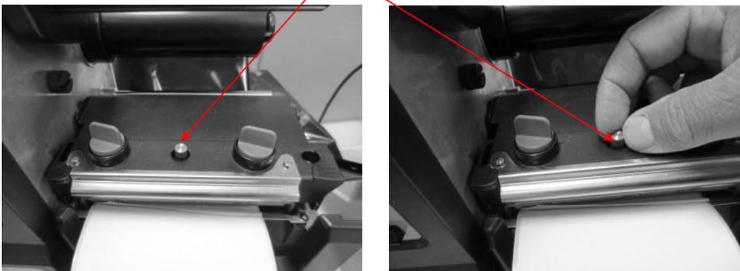
5. Push the deck lock lever to release the pivoting deck.
