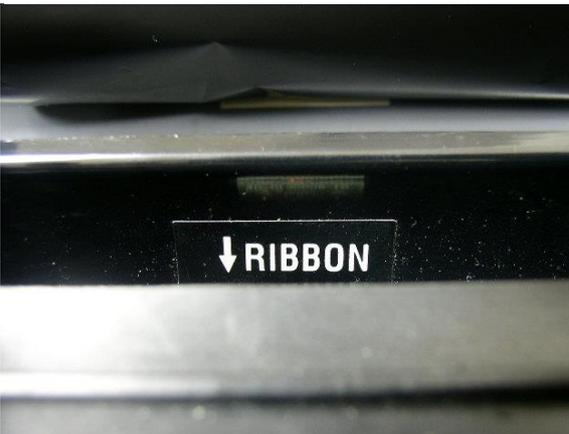
7. Following the direction of the ↓ **RIBBON** label, pull the transparent ribbon leader to the front from under the ribbon mechanism.
