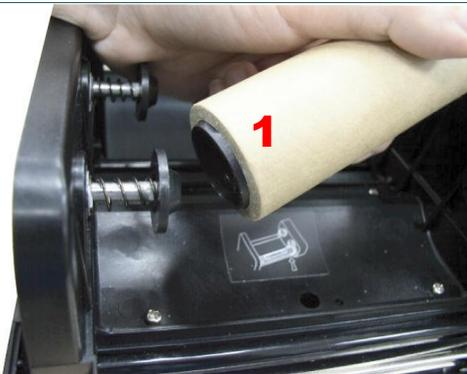
2. Insert the left side first. Mount the ribbon rewind paper core on the front hubs.
