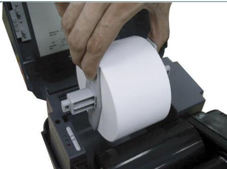
4. Place the label roll into the label roll mount/ or external label roll mount. Feed the label under the carriage and over the platen.
