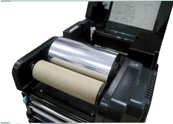
5. Please be noted that the bigger hub side with 4 ribs must be installed toward the right side of ribbon mechanism.
