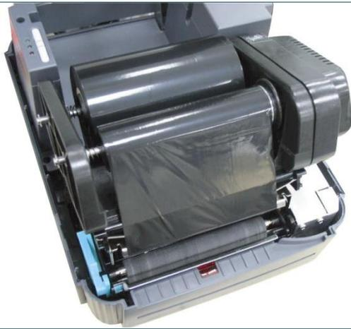
9. Rotate the ribbon rewind spindle until the ribbon overlaps the ribbon leader and stretches tight.
