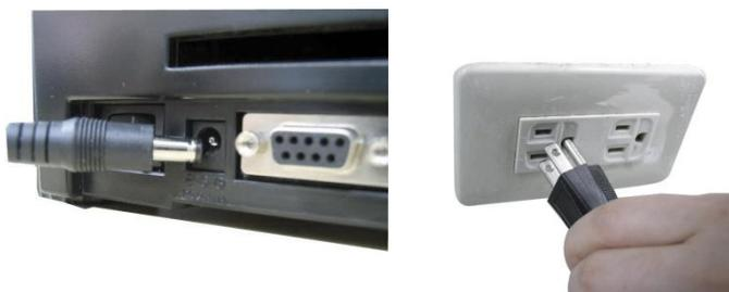
4. Plug the power cord into the power jacket at the rear of the printer, and then plug the power cord into a properly grounded receptacle.
