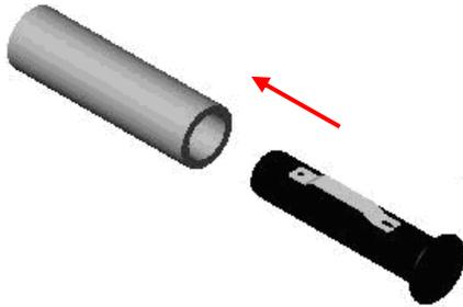
1. Place an empty paper core on the ribbon rewind spindle.
