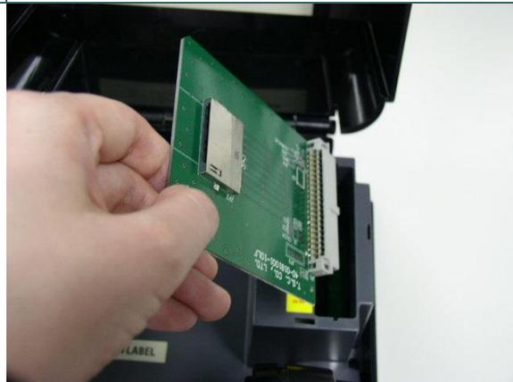
2. Plus the SD memory card module on the main board.
