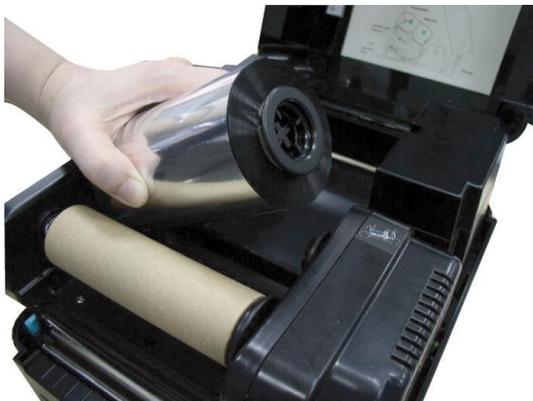
4. Install a ribbon on the ribbon supply spindle. Mount the ribbon supply spindle on the rear hubs.
