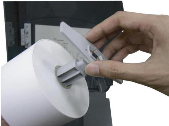
3. Slide the label supply roll spindle through the core of a label roll and attach the fixing tabs onto the spindle.
