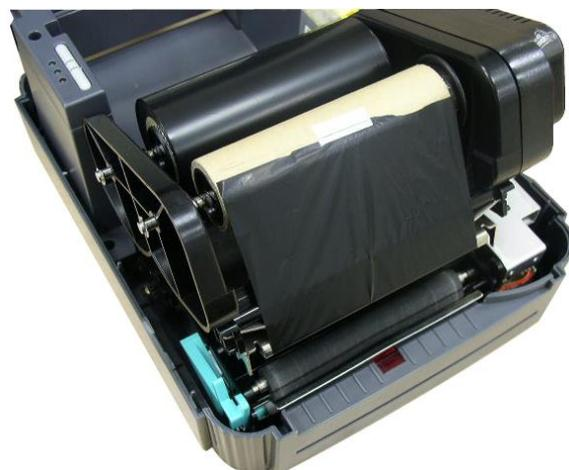
8. Attach the ribbon leader to the empty paper core on the ribbon rewind spindle (with a tape).
