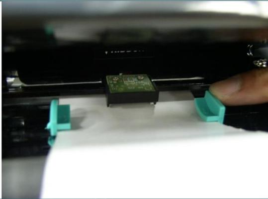
5. Adjust the label guide to fit the width of the media.
