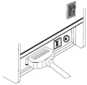
Plug the cable connector securely into the printer's interface connector.
